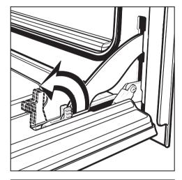
Slowly shut the door until the protruding clamps stop the movement. Pull the door upward. See illustration.
